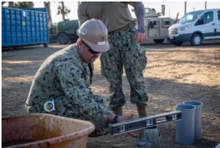
Equipment Operator 1st Class William Price, a Seabee assigned to Naval Mobile Construction Battalion (NMCB) 5, levels a slump cone during a field training exercise (FTX) onboard Naval Base Port Hueneme
